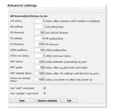
**NOTE 4:** Some CAM have a high initial power consumption. If one see problem at startup, change the "Power on startup delay to value 45000 for CAM 1 and 50000 for CAM 2.
